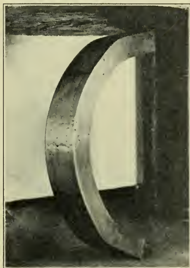
FIGURE 5—End of the Free Bend Test, showing the stretching to which the metal in the weld has been subjected.
